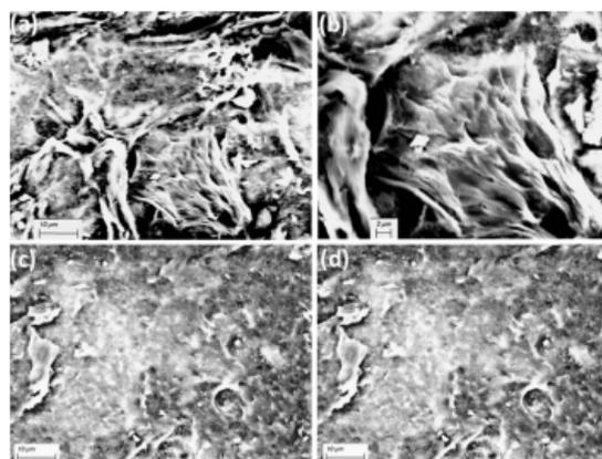
**Fig. 8** The scanning electron micrographs of zirconium alginate biosorbent before fluoride uptake, at (a) 10 μm and (b) 2 μm; after fluoride uptake, at (c) 10 μm and (d) 2 μm scale.
