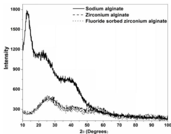
**Fig. 6** The XRD pattern of biosorbents sodium alginate, zirconium alginate and fluoride sorbed zirconium alginate.
