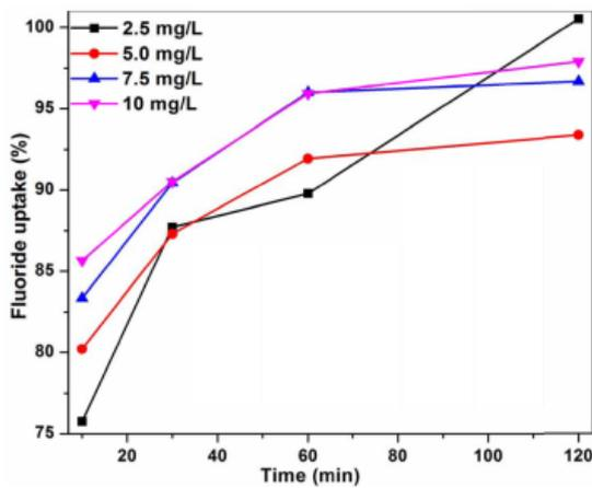
**Fig. 3** The time dependent fluoride uptake by the biosorbent at pH 5 and varying initial fluoride concentration.
