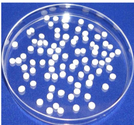
**Fig. 1** The digital photograph of zirconium alginate biosorbent beads.
