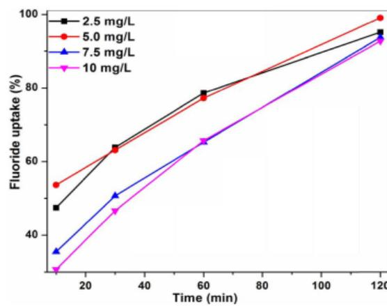
**Fig. 4** The time dependent fluoride uptake by the biosorbent at pH 7 and varying initial fluoride concentration.
