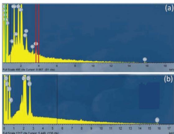
**Fig. 9** The EDX spectra of (a) native and (b) fluoride sorbed zirconium alginate biosorbent.
