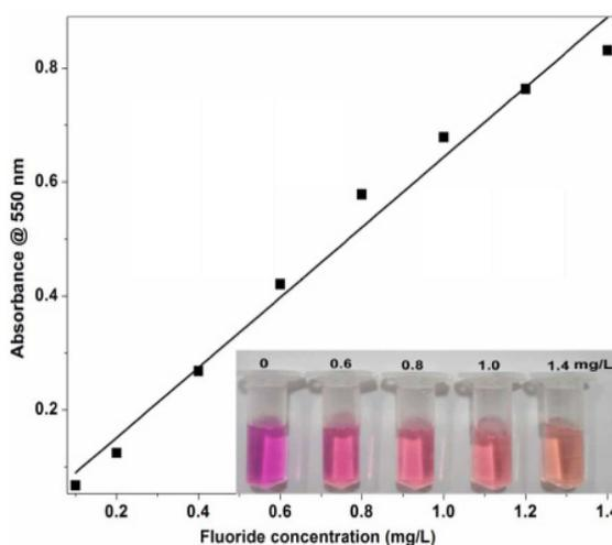
**Fig. 2** The calibration plot showing the absorbance at 550 nm vs. fluoride concentration. Inset: Solution colour at various fluoride levels.
