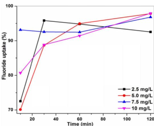
**Fig. 5** The time dependent fluoride uptake by the biosorbent at pH 9 and varying initial fluoride concentration.
