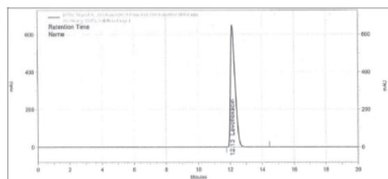
**Fig. 2.2.** Accuracy (Spike level 150%) chromatogram
