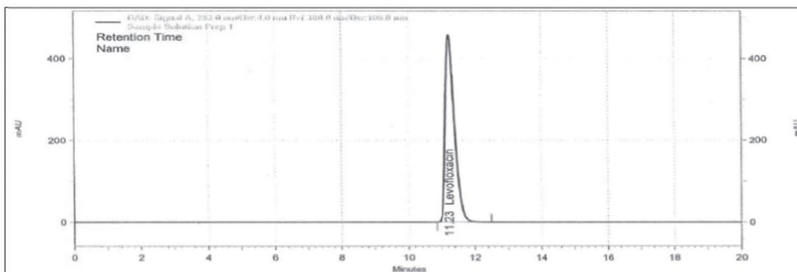
**Figure: 1.6.** Method precision sample chromatogram
