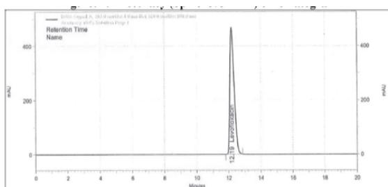
**Fig. 2.0.** Accuracy (Spike level 100%) chromatogram
