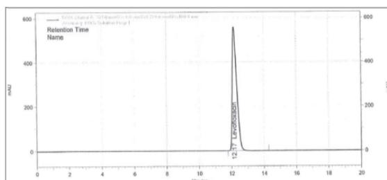
**Fig. 2.1.** Accuracy (Spike level 125%) chromatogram
