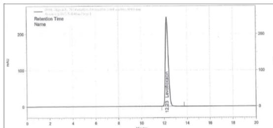
**Fig. 1.8.** Accuracy (Spike level 50%) chromatogram
