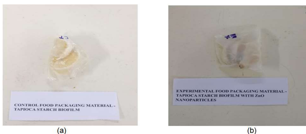
Figure 3: (a) F1 film wrapped over sweet lime segments, (b) F2 film wrapped over sweet lime segments- post 28 days stored at 4°C
