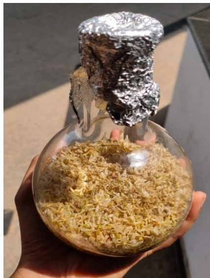
Fig 1. Shade dried Neem flowers soaked in ethanolic extract in round bottomed flask
