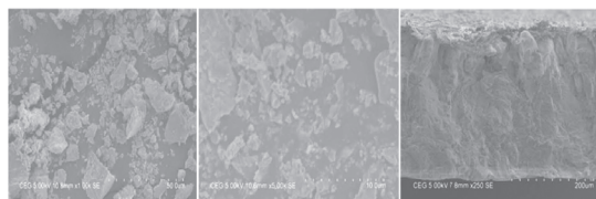
Figure 7 : SEM Image of egg shell, particle's shape and size changed with calcination with different temperatures and time
