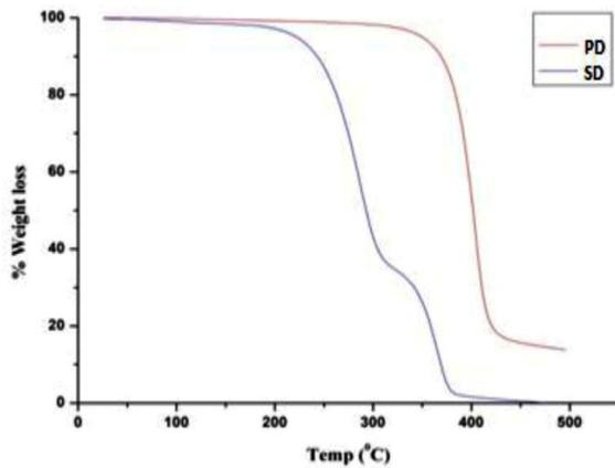
**Figure 6:** Comparative TGA graph of Pure drug (PD) and optimized solid dispersion
