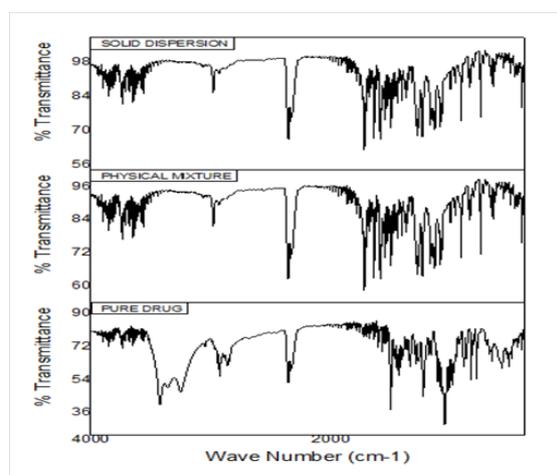
**Figure 2:** Comparative FT-IR spectra of Pure drug (FENO), Drug + HPMCAS (PM) and Optimized SD
