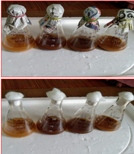
Figure 1 (a): The Fungal substrate of DDT degrades 7d incubation (b) The fungal substrate of DDT degrades 28 d incubation.
