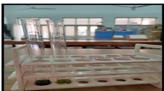
Fig. 8: Azadirachta indica n-hexane extract Steroid test Indicating test -negative no red color
