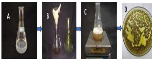
Fig. 1: Synthesis of zinc nanoparticle (A) Preparation of zinc sulphate chemical (B) Plant extract + zinc sulphate (C) Magnetic stirrer for 2 hours (D) Synthesis of zinc sulphate nanoparticle
