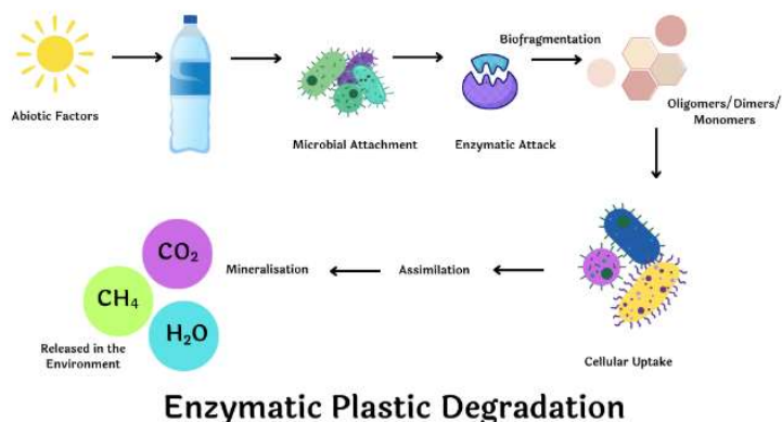
Fig. 4: Degradation of plastic waste through enzymatic process
