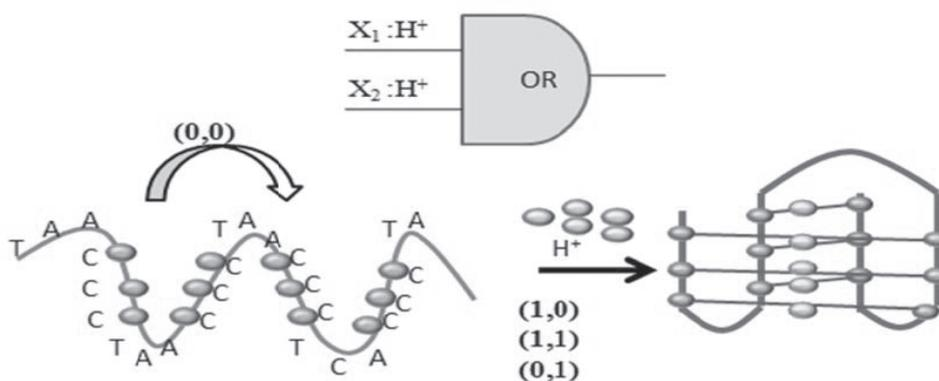
**Fig 6.** Demonstration of OR gate.
