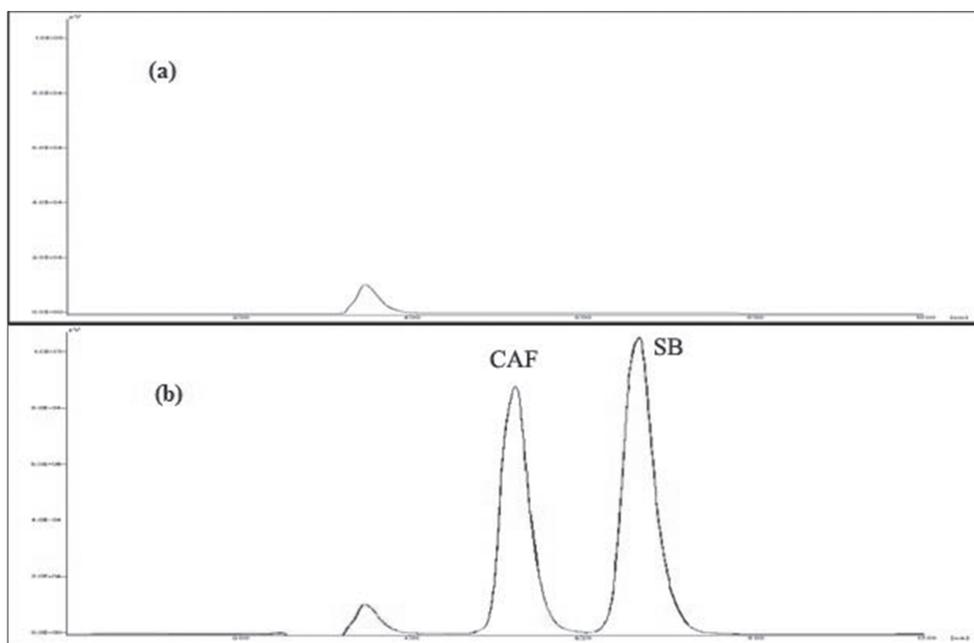
Fig. 3. (a) Blank (b) Chromatogram of caffeine and sodium benzoate
