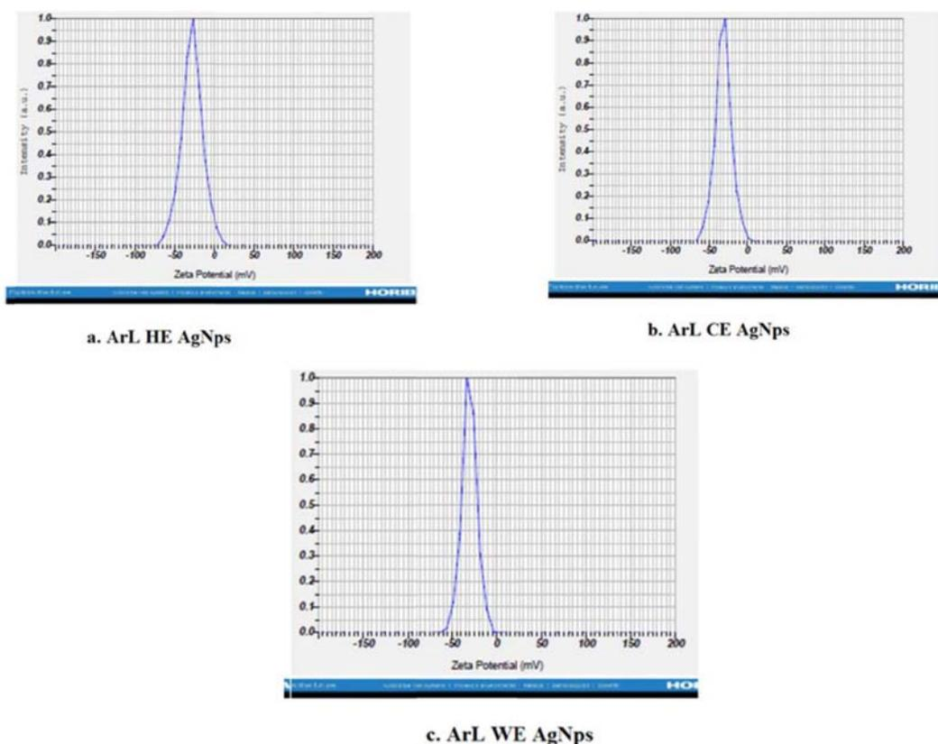
**Fig. 4.** Zeta potential of AgNPs synthesized by fractionated *A. reticulata* leaf extract in different solvent. (a) Hexane extract AgNPs (b) Chloroform Extract AgNPs (c) Water extract AgNPs.
