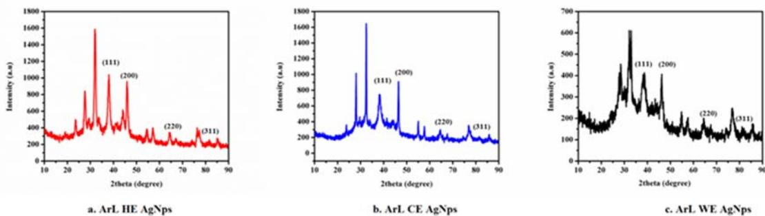
**Fig. 6.** XRD pattern studies confirming the crystal nature of the AgNPs by showing the Bragg's peaks corresponding to (111), (200), (220) and (311) planes of (a) *A. reticulata* Hexane Extract AgNPs (b) *A. reticulata* Chloroform Extract AgNPs (c) *A. reticulata* Water Extract AgNPs.
