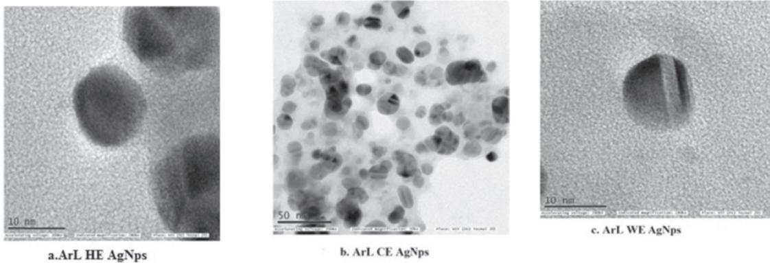
**Fig. 7.** Shows TEM micrograph of synthesized AgNPs in different solvent fractionated *A.reticulata* Leaf extracts. (a) *A.reticulata* Hexane Extract AgNPs (b) *A.reticulata* Chloroform Extract AgNPs (c) *A.reticulata* Water Extract AgNPs.
